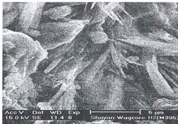
Figure 7 Crystalline (Rosette) AAR products in the white reaction rims seen within the aggregate boundaries
